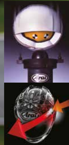
All helmets protect the rider's head through both glancing off and energy absorption.
