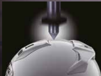
The helmet penetration test drops a 3kg striker onto the helmet from 3 meters up. The test confirms the strength of the helmet against failure from the road surface, obstacles in the road, footpegs, or other potential hazards.
