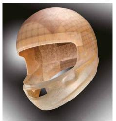
The top of the eye port has a Super Fiber Belt which reinforces the helmet like the bands of a barrel for better protection. This special belt suppresses the spreading of cracks that form when the helmet receives a large impact and improves glancing off.
