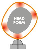
The head form shape used in helmet testing is somewhat square, so the 'four corners' get tight inside the helmet, and we can see a tendency to make the shell square too.
